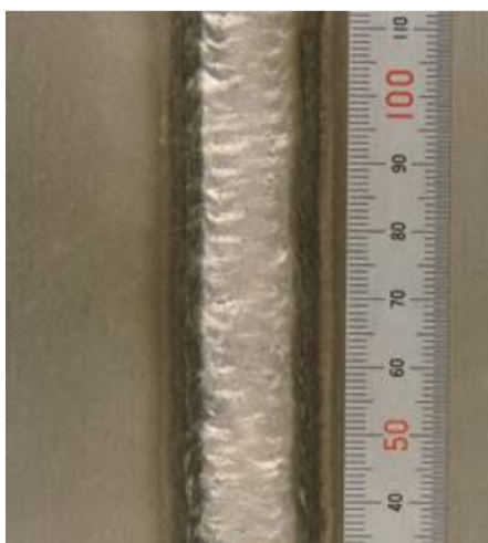
Wire: PREMARC DW-2594 Base Metal: S32760, 3/4" Vertical-up (3G)
