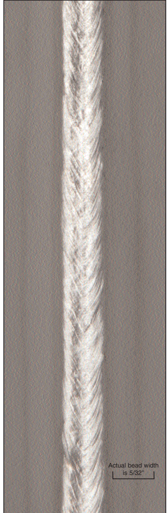
Fig. 1- Horizontal fillet in 120A-22V (100% CO 2 ) with DWG-308L. Stable arc transfer and ideal slag formula.
