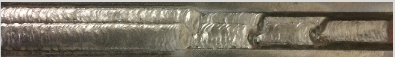
DW-50, 0.045", vertical upward welding at 64kJ/in with mixed gas
