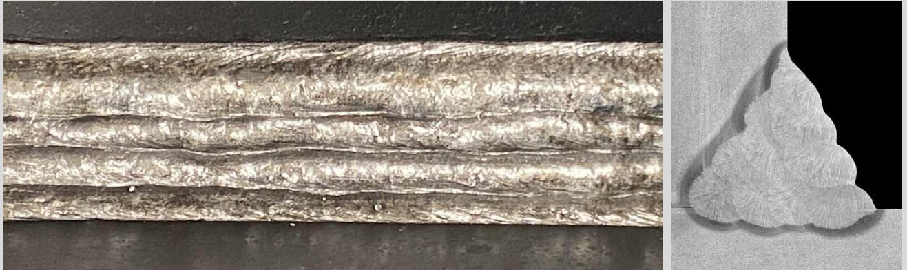
DW-50AY, 3/32", Horizontal Fillet Welding at 43.2kJ/in with 100%CO 2 gas
