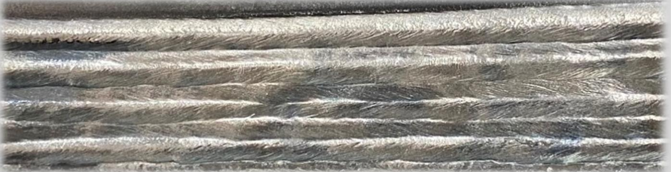
MX-50R, 0.052", Horizontal Groove Welding with ARCMAN™ series Portable with 100%CO 2 gas
